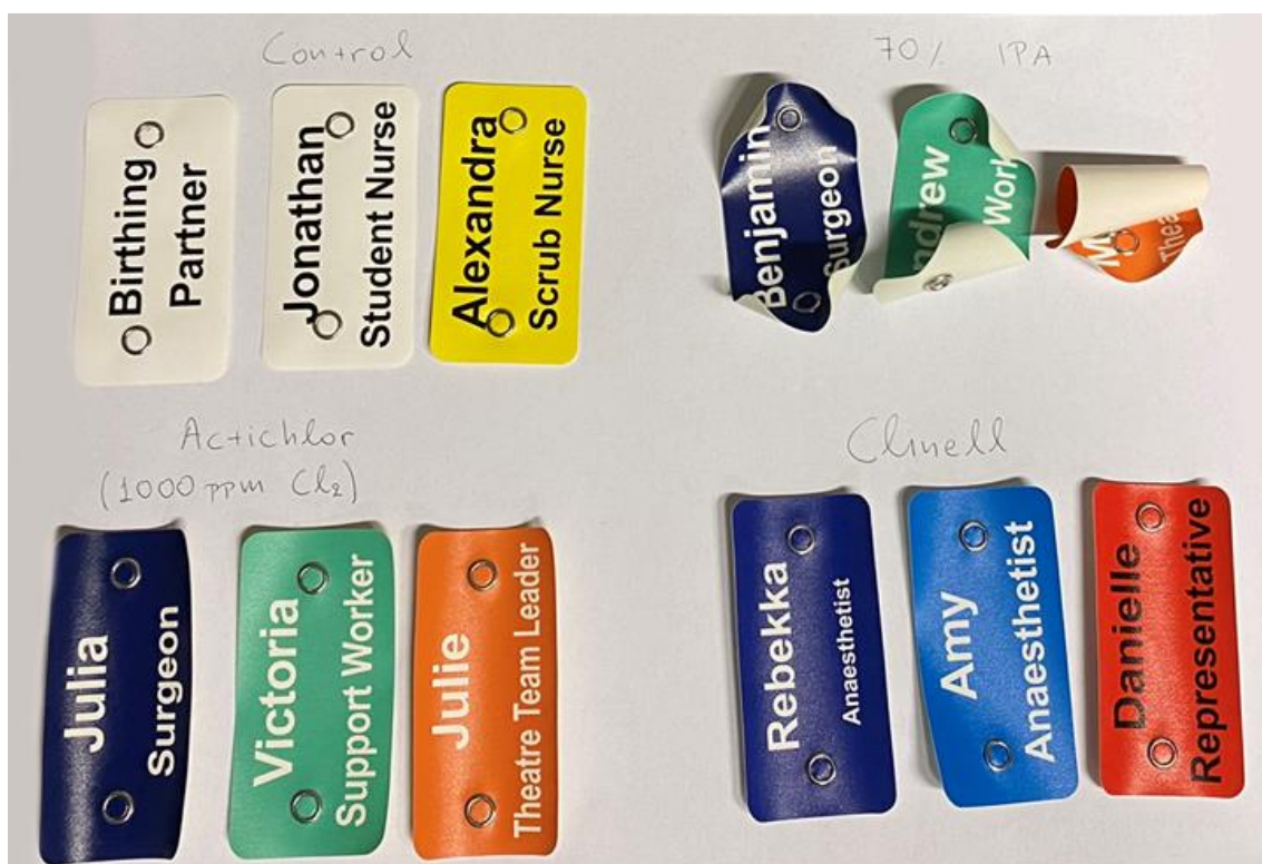
Figure 9: Front side of the polyester badges, post the chemical degradation experiment.
