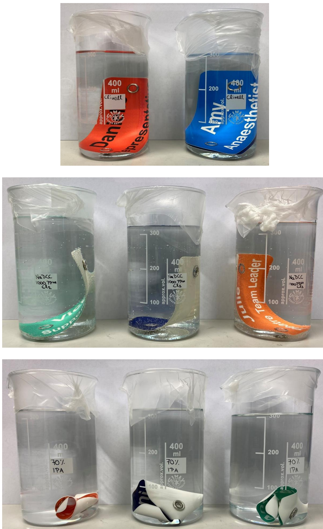
Figure 8: Clinell (up), Actichlor (mid) and 70% IPA (bottom) test groups, post the chemical degradation experiment.
