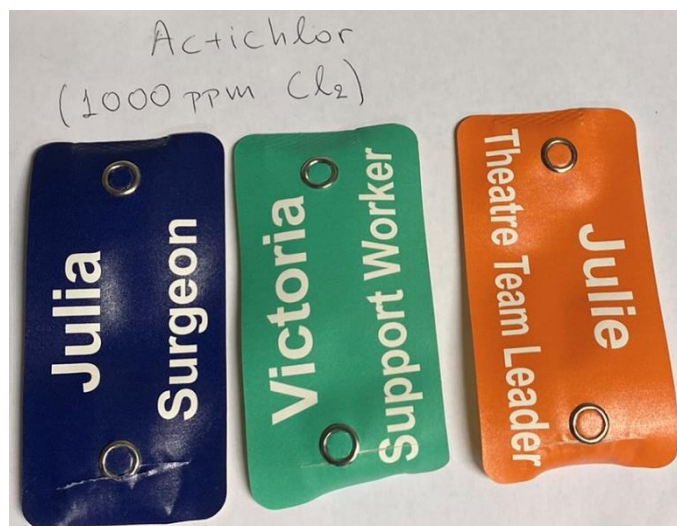
Figure 15: Front side of the polyester badges, post the tensile strength tests.
