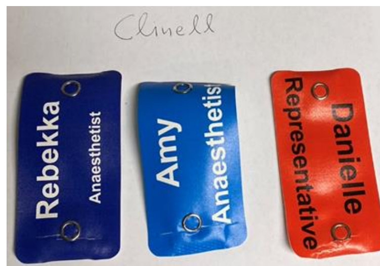
Figure 15: Front side of the polyester badges, post the tensile strength tests.
